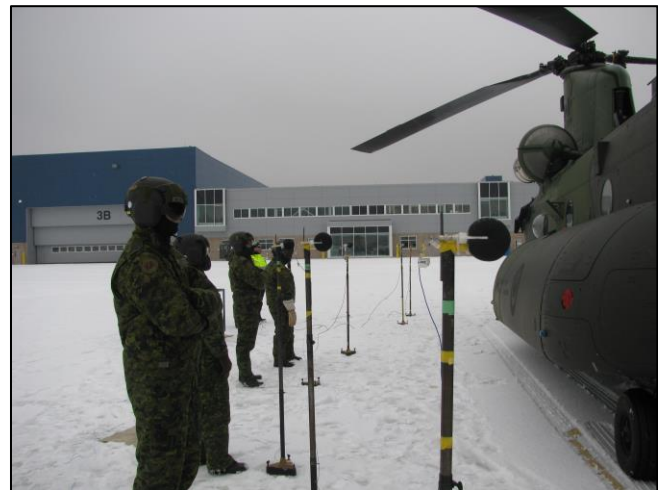
Figure 2: Exterior Noise Measurement
