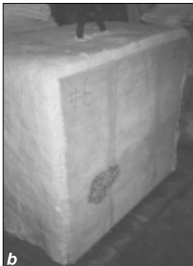
Figure 5. View of high-strength concrete blocks after two-hour hydrocarbon fire test: (a) block without polypropylene fibres; (b) block with polypropylene fibres
