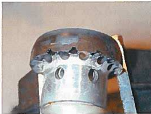
Fig.12: Damaged fuel nozzle swirler.
