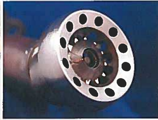
Fig.13: Laser clad repaired fuel nozzle swirler after final machining.
