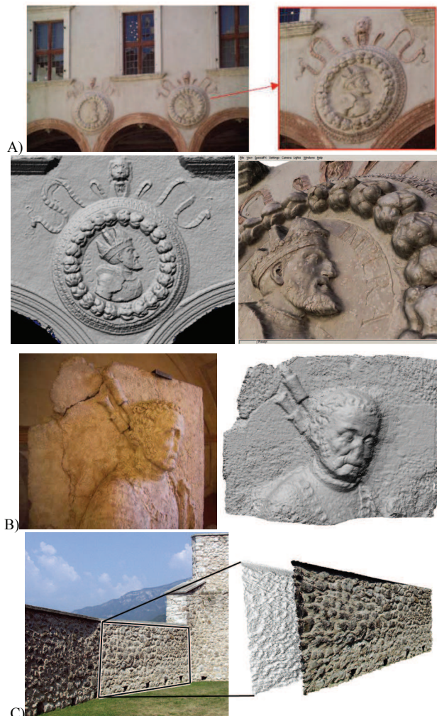
Figure 4: Detailed models achieved with multi-photo matching (A and B) or Depth from Shading (C).
