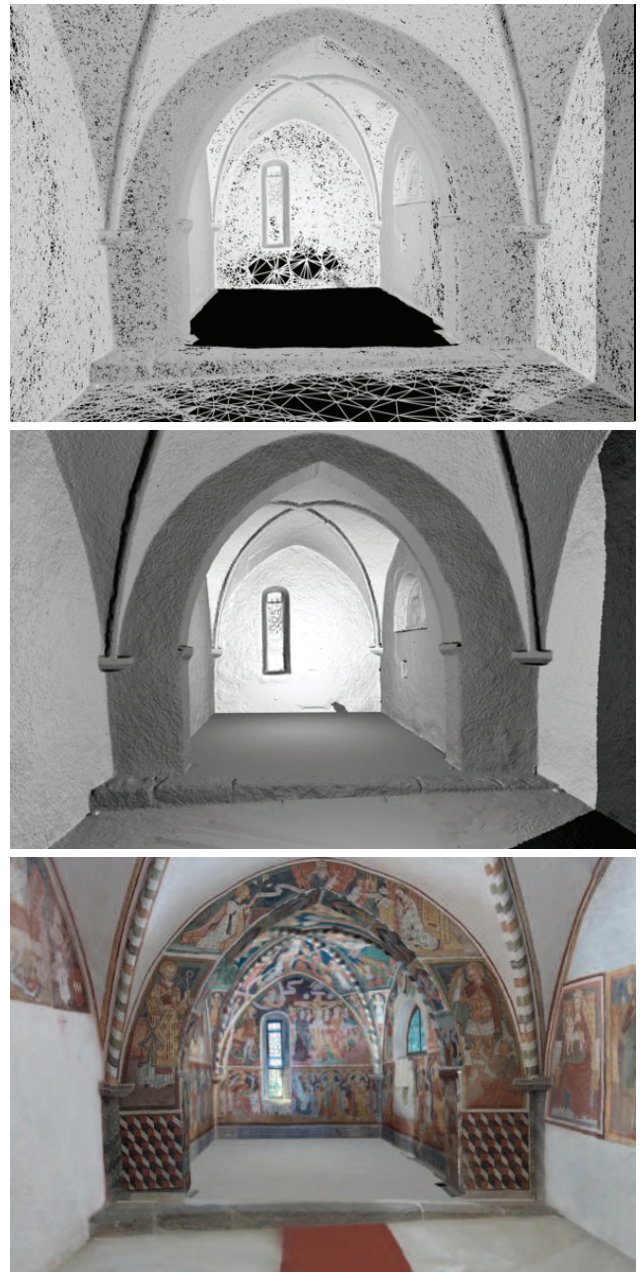
Figure 6: Wire-frame, shaded, and textured model of an interior chapel altar in the Valer castle.
