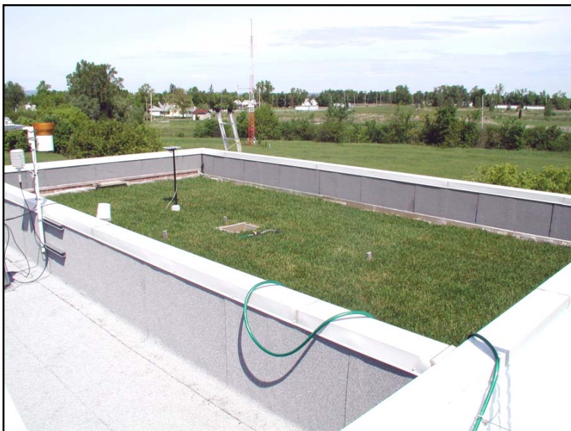
Figure 4 The sod two weeks after installing on the FRF in the NRC campus in Ottawa (2002). Note that the median divider separates the Green Roof (left) and the Reference Roof (right). The weather station is located at the median divider.
