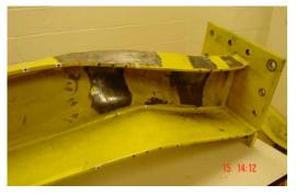
Figure 20 Tee-75 end load test.
