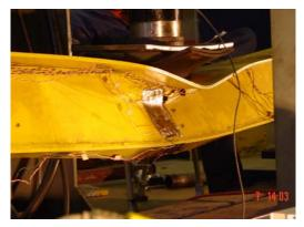
Figure 18. Tee-75 central load test.
