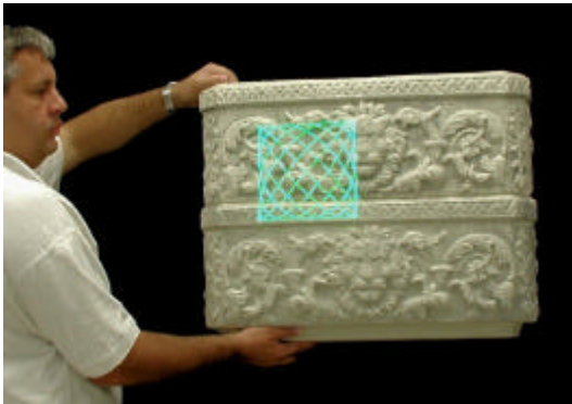
Figure 5: Demonstration of hand-held acquisition using fast scanning patterns and real-time 3D tracking. The use of external positioning devices is not a solution because they can't be fixed to the object. No external equipment is needed eliminating the constraints imposed by mechanical rigidity and stability during the acquisition.
