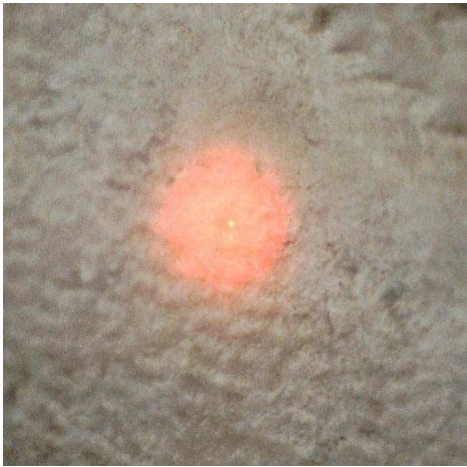
Figure 6: Subsurface scattering on Michelangelo's Bearded Slave . The visible halo around the laser spot is 2 cm approx.
