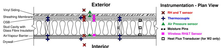
Figure 2. Plan view of wall cross section
