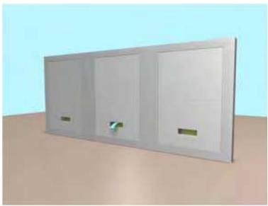
Sits in air barrier and wood sheathing allow exfiltration and infiltration.
