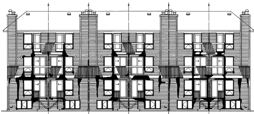
Figure 3. Pattern of distribution of the damage to the exterior sheathing board (Project A)
