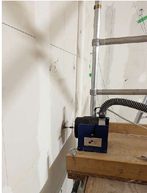
Figure 4: Shaker attached to one of the timber framed walls via an impedance head.
