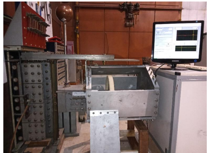
Fig. 2. A photo of the calibration system with the hexagonal coaxial cage.
