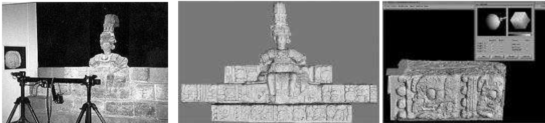
Figure 4. The Biris 3D Laser Camera (left) is shown mounted on a linear translation stage scanning a section of the Hieroglyphic Stairway at the Peabody Museum. The Stairway measures approximately 3.4 m wide and is approximately 2.3 m at its highest point. The complete 3D model is shown in the center. The artificial shading feature of the software can be used to study the writing on any section of the model (right).
