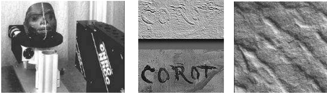
Figure 1. The High Resolution Color Laser Scanner (left) imaging the Tsimshian Stone Mask from the Canadian Museum of Civilization. In this configuration, the scan is made by rotating the mask 360° on a rotation table. The scanning mechanism projects a white laser spot (white line profile) on the mask from a RGB laser. Details of a Corot signature (center) and tool mark features on one of Michelangelo's Prisoner sculptures in Florence (right).
