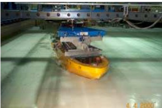
Fig. 7 The PMM Terry Fox Model Test (Lau, 2006)
